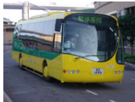
Figure 3: Hybrid diesel/electric Shuttle Bus
