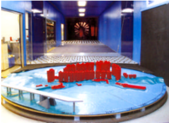
Figure 4 : Wind Tunnel Modelling for enhancing Pedestrian Comfort
