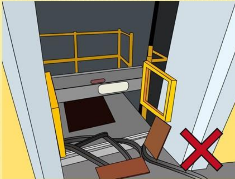
Poor Housekeeping at the access 升降机槽出入口欠妥善整理
