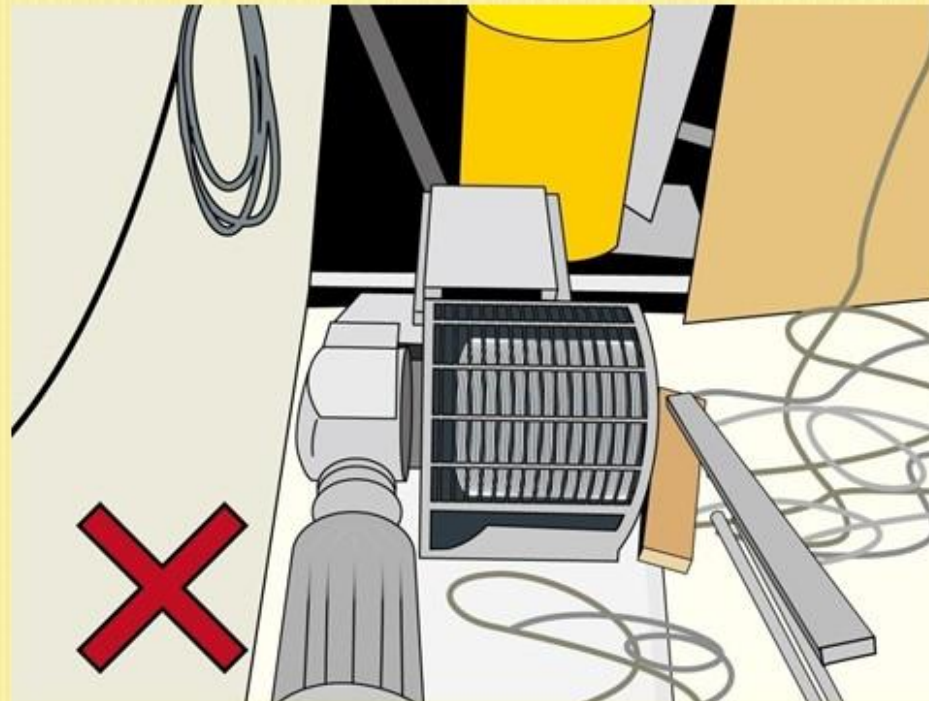
Improper Guarding on Electrical Winch 电器绞盘保护不当
