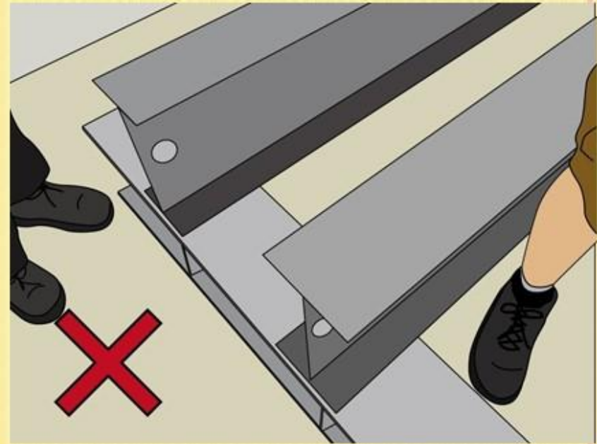
Sharp edges of H-beams in lift machine room should be adequately protected. 在电梯机房的锋利的边缘应得到充分保护。
