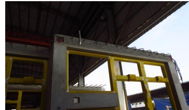
Concealed Conduits and Equipotential Bonding Accessories in Precast Elements
