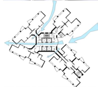
VENTILATED LIFT LOBBY
