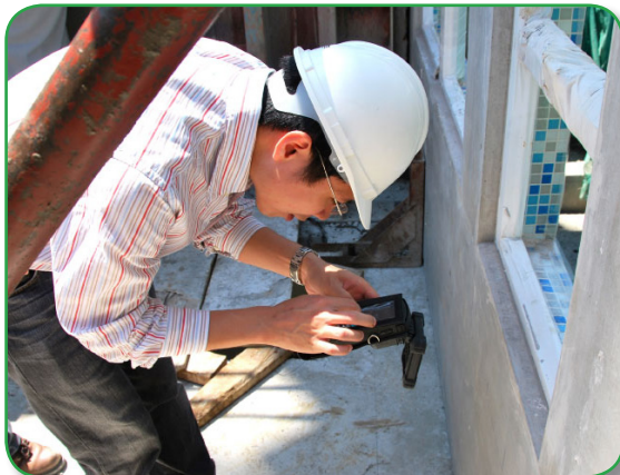
Read/write data using the Radio Frequency Identification reader on the embedded tag
