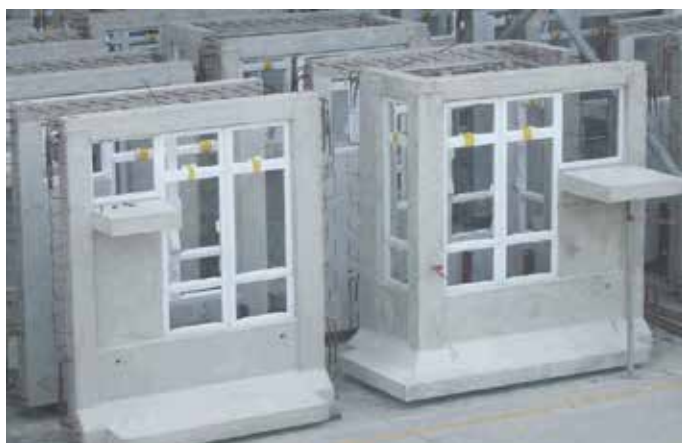
5 Close-up of GGBS (left) and GGBS used in the construction of precast concrete façades
