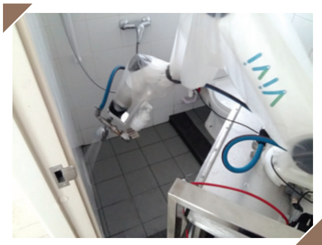
A robot conducting water test at bathroom
