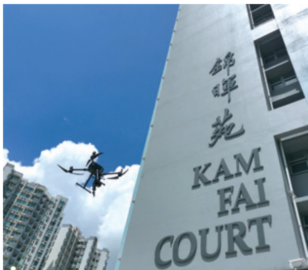
無人機在檢測外牆 UVA inspects external walls of a block
