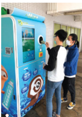
設置於梨木樹邨的逆向自動售貨機 A reverse vending machine placed at Lei Muk Shue Estate
