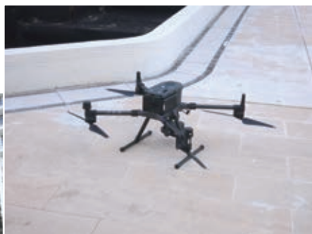
无人机在海达邨检测外墙 SUAs camera inspects external wall in Hoi Tat Estate
