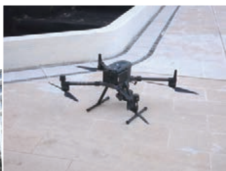
無人機在海達邨檢測外牆 SUAs camera inspects external wall in Hoi Tat Estate
