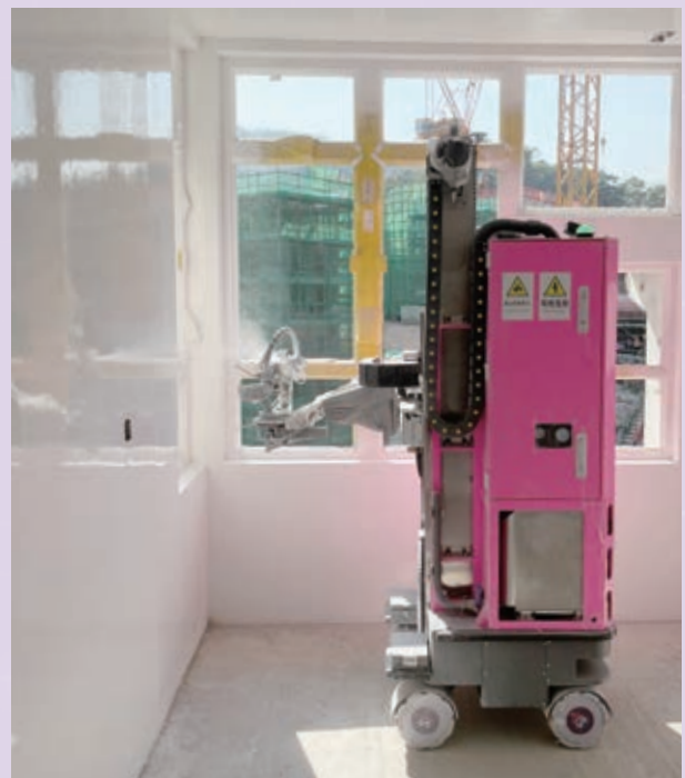
在公營房屋項目中試用油漆機器人 A painting robot trial in a public housing project
