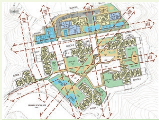
大埔富蝶邨善用布局，在住宅大厦间留下通风走廊，加强自然通风 The domestic blocks at Fu Tip Estate, Tai Po are positioned to form open breezeways for better natural ventilation
