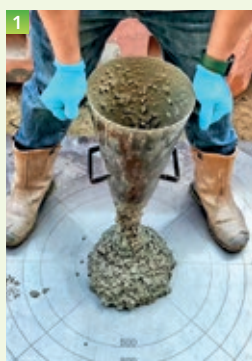
我们的合作研发机构在先导计划的试验桩应用粒化高炉矿渣粉前，就不同配比的矿渣粉混凝土配方进行测试（左起） Our collaborative research institute conducted tests on different GGBS concrete formulations (from left) before applying GGBS to the test piles of a pilot project
