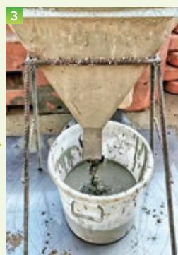
我們的合作研發機構在先導計劃的試驗樁應用粒化高爐礦渣粉前，就不同配比的礦渣粉混凝土配方進行測試（左起） Our collaborative research institute conducted tests on different GGBS concrete formulations (from left) before applying GGBS to the test piles of a pilot project
