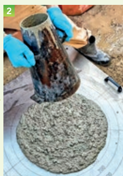
我們的合作研發機構在先導計劃的試驗樁應用粒化高爐礦渣粉前，就不同配比的礦渣粉混凝土配方進行測試（左起） Our collaborative research institute conducted tests on different GGBS concrete formulations (from left) before applying GGBS to the test piles of a pilot project
