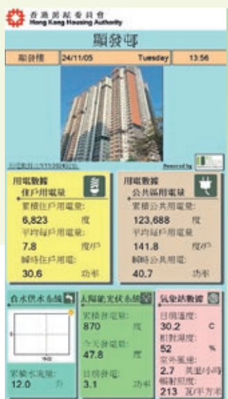
智能計量儀監察系統 A Smart Meter Monitoring and Energy Information Display System
