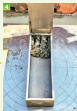
我們的合作研發機構在先導計劃的試驗樁應用粒化高爐礦渣粉前，就不同配比的礦渣粉混凝土配方進行測試（左起） Our collaborative research institute conducted tests on different GGBS concrete formulations (from left) before applying GGBS to the test piles of a pilot project
