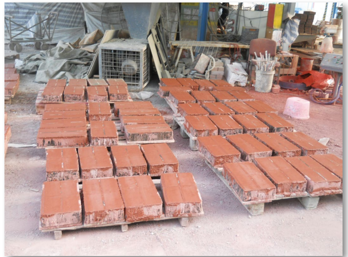
Paver blocks made of cement-stabilised marine mud
