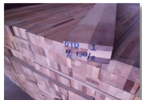
Composite joints in timber doorsets
