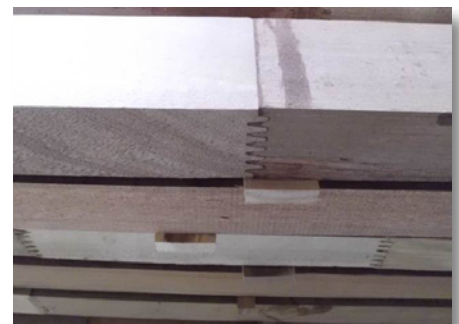
Finger joints in timber doorsets
