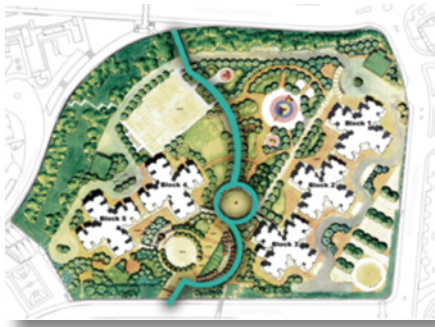
Building setback to reduce noise at receiver end
