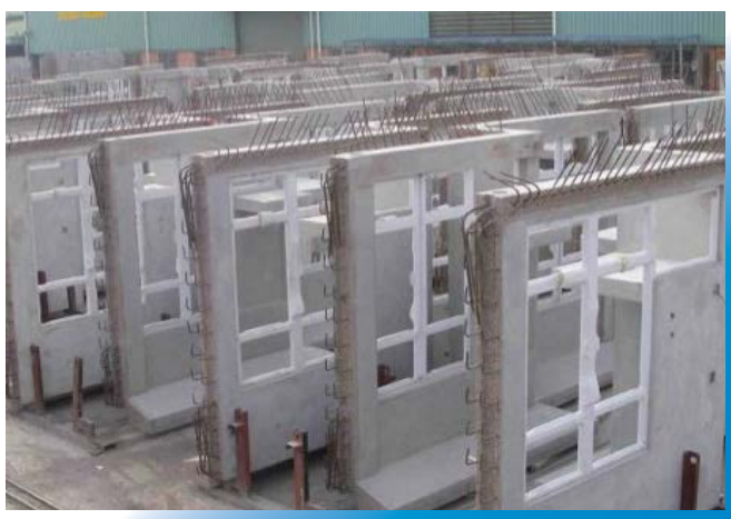
▲ Precast Façades with GGBS
