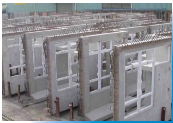
▲ Precast Façades with GGBS
