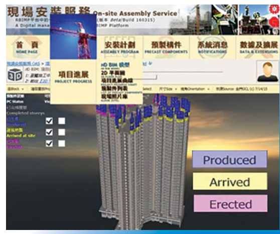
▲ BIM Model in Web-based Operating Platform - nD BIM Showing Façade Installation
