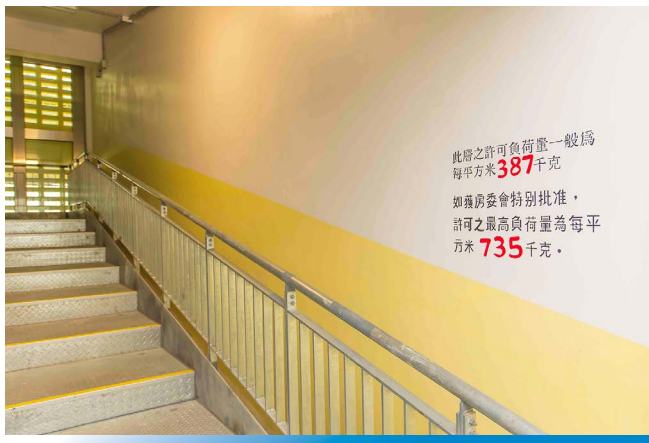
▲ Floor Loading Capacity
