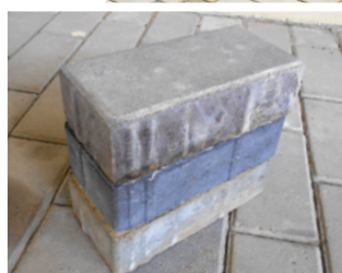
▲ Use of recycled glass cullet as aggregates for precast concrete paving blocks (top and bottom)
