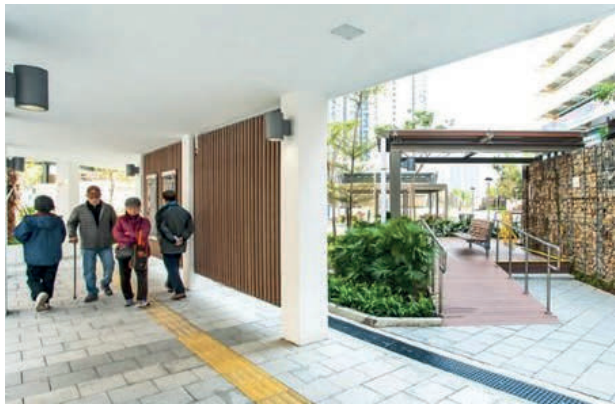
Ramps and tactile paths at external area to enhance accessibility
