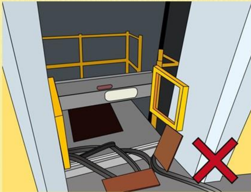
Poor Housekeeping at the access 升降機槽出入口欠妥善整理
