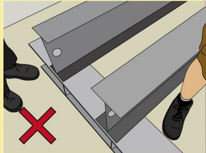
Sharp edges of H-beams in lift machine room should be adequately protected. 在電梯機房的鋒利的邊緣應得到充分保護。
