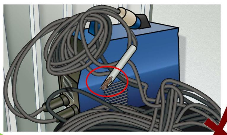
Damaged earthing connector for arc welding machine 電焊機接地線損壞
