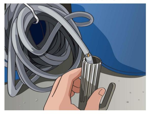
Damaged welding holder 損壞的燒焊鉗
