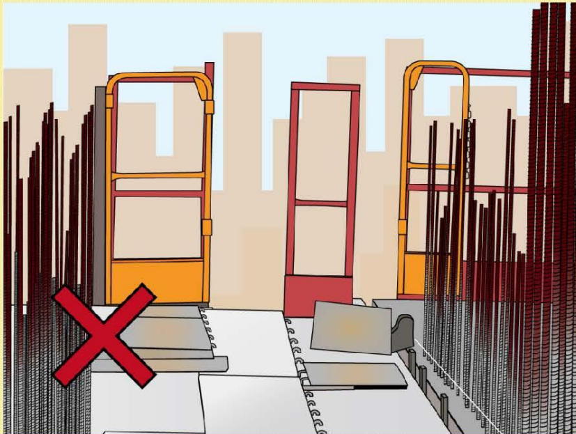
Guard-rail on Working Platform at Wall Form Panel not Securely Closed 工作台圍欄未有鎖好
