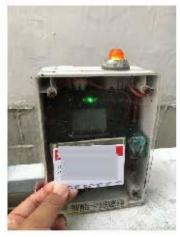
In order to effective control of competent operators, a RFID system was in place. The authorized worker must use the RFID card together with the key in order to operate the gondola / enter into the lift shaft.
