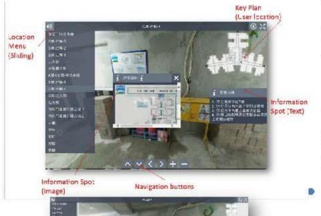
The mobile platform provides interactive menu and buttons where users are able to navigate from first person perspective through out all the preset site locations/spots.
