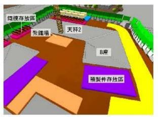
The BIM site facility layout displayed different work areas on the construction site. Through BIM, it can be used in the induction training course and allow better understanding for new coming workers.
