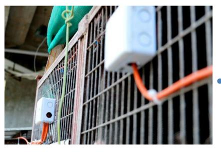
The new infra-red interlock requires both gates to be closed properly to activate hoist movement. The hoist movement will be deactivated when the new infra-red interlock was being interfered.
