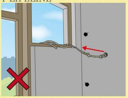
如果側身負載,吊環螺栓可能會彎曲。麻袋應放在周圍鋒利的邊緣/角以保護救生繩。If the load is applied sideways, the eyebolt may bend. Sacking should be placed around sharp edge/corner to protect the lifeline.
