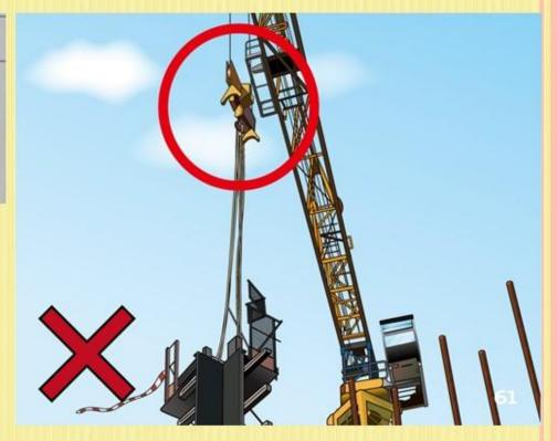
鈎環的方向不正確 - 鈎環杆應經常扣在吊鈎上 鈎環尺寸過小,引致鈎環的方向錯誤 The Orientation of Shackle was wrong - The Jaw OF THE HOOK SHOULD FIT AROUND THE PIN OF SHACKLE. The Size of Shackle Seems too Small and This May LEAD TO THE WRONG ORIENTATION OF THE SHACKLE
