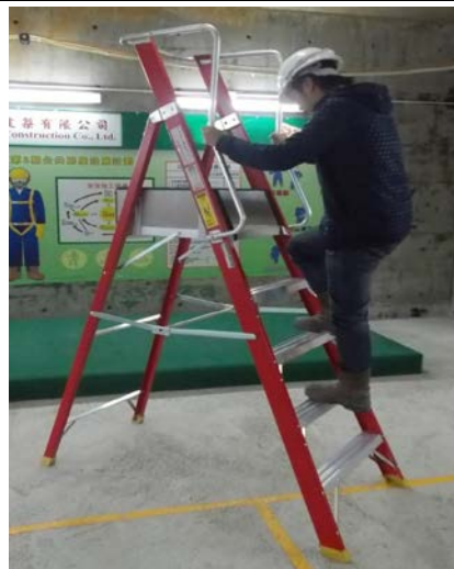
Platform ladder with platform at more than 900mm but less than 2m from floor level
