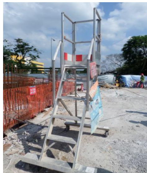
Platform ladder with platform at more than 900mm but less than 2m from floor level
