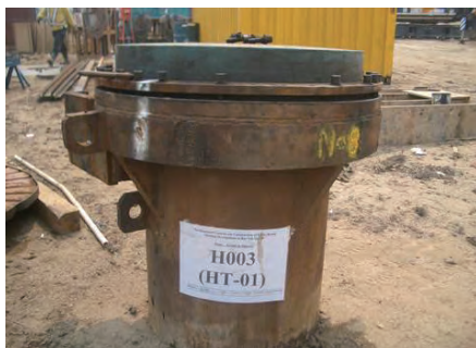
整个打桩过程须使用胶垫以减少噪音 Plastic cushion to reduce noise generated during the course of piling
