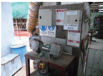
为砂轮机设置护罩和在当眼处张贴安全海报／告示 Abrasive wheel with guarding and relevant notice/poster is posted at the location
