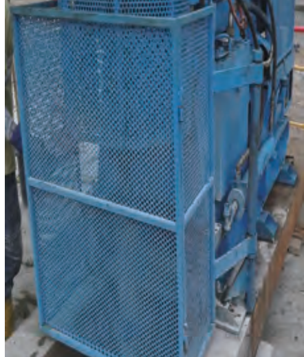
钻机的活动部分必需设置护罩 Moving part equipped with shield guard
