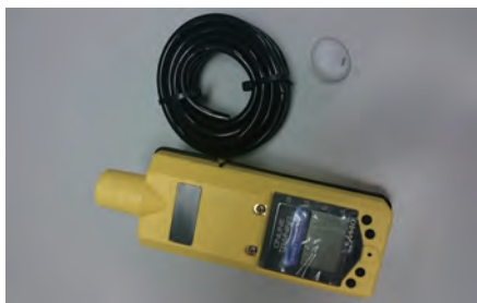
使用经过校准的气体探测器量度密闭空间内有毒／易燃气体的浓度 A calibrated gas detector used to measure the concentration of poisonous/flammable gases inside a confined space
