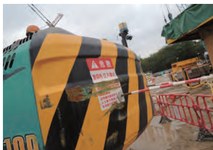
在挖土机尾部安装闭路电视摄影机 CCTV installed at the rear part of Excavator
