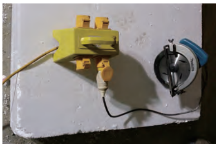
降压变压器将高压电降低至110伏特，适合一般手提电动工具使用 Step-down transformer provides 110V power supply source for use by hand-held tools
