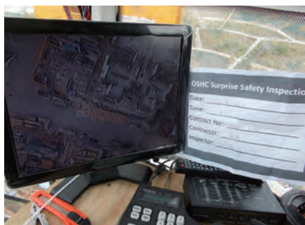
塔式起重机操作员藉闭路电视屏幕监察吊运区情况 CCTV system helps the tower crane operator to monitor the situation of lifting area
