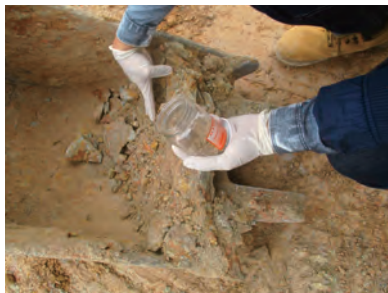
拆卸工程前，应取样检验怀疑受污染的土壤：受污染的物质必须被移离 Prior to demolition, soil sample should be collected/ tested and the contaminated soil must be removed
