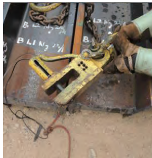
可扣紧工字桩末端的特制起重装置 Lifting gear tailor designed to clip the end of H-pile
