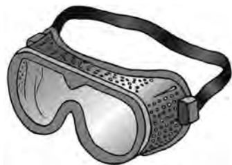
(附透气孔·不适合腐液及烟雾) (Goggles with direct vents are not suitable for protection from chemical splattering or smoke)
