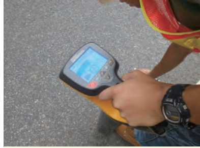
以手提探测器检测地下公共设施的走线及其位置 Hand-held detector to check routing and locate for underground utilities
