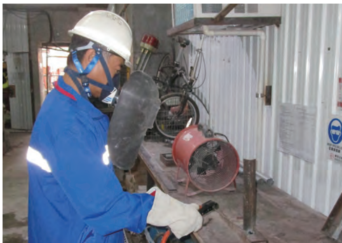
焊工穿上个人防护装备方可进行焊接工作 Welders with personal protective equipment during welding
