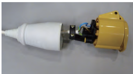
插座内的电线应妥善接驳于接线座，电线不得外露 Properly connect wiring in the socket and no live conductor exposed from the termination block
