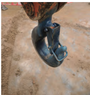
为吊钩的安全扣加装保险扣 Additional safety lock is added to the safety latch of hook
