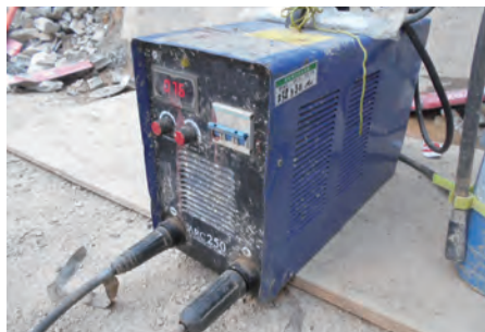
焊机壳必须接地（带电部份需要有绝缘保护） Shield of welding machine - Earthed (Live conductor terminals should be insulated)
