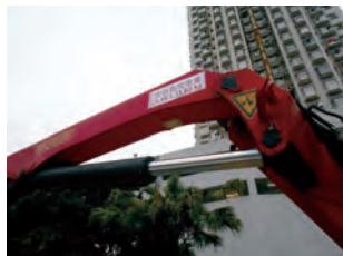
起重机上清楚标示安全操作负荷 Safe working load clearly marked on the crane
