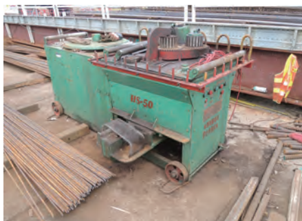
屈曲钢筋机器需有足够的工作空间 A typical steel bending machine on site with adequate working space
