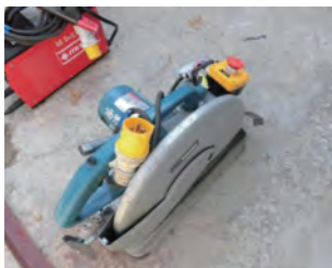
风车／圆锯应设有护罩和紧急停止掣 Circular saw with guard and emergency stop
