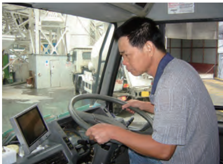
安装闭路电视及萤光幕让驾驶员清楚看见车辆后面的交通情况 Install CCTV and monitor for driver to have view of traffic at rear of vehicle
