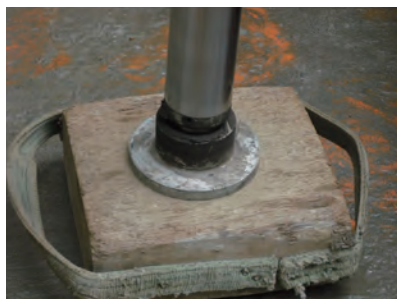
起重垫板的面积不得小于支重脚撑踏板面积的三倍 The lifting mat of area not less than 3 times of the float of the outrigger leg
