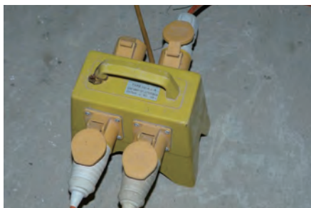
降压变压器将高压电降低至110伏特，适合一般手提电动工具使用 Step-down transformer provides 110V power supply source for use by hand-held tools
