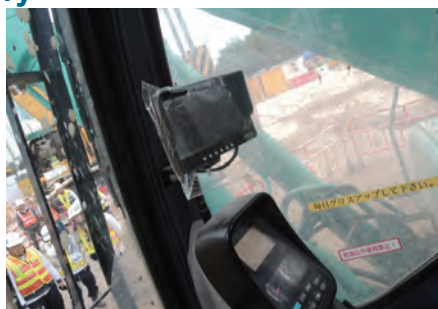
操作员透过闭路电视可观察四周情况 Install CCTV system for operator to have a clear view of surrounding
