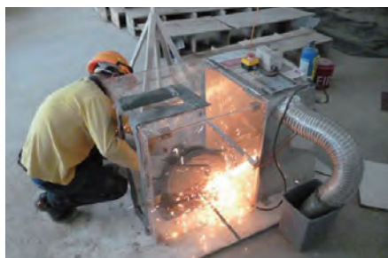
为割碟机安装隔音和隔尘保护罩 Sound insulation and dustproof protection guard provided to abrasive cutter
