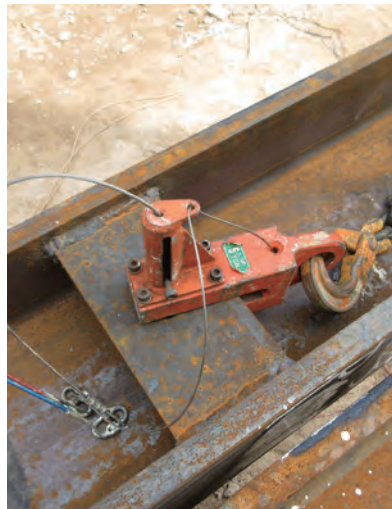
专为吊运字H字板桩用途的吊具 Tailor-made lifting gear for H-beam
