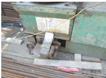
屈曲钢筋机器需设置的护罩 Bar bending machine with guarding
