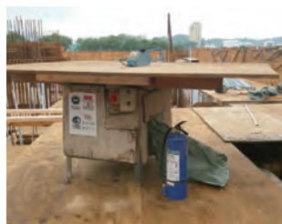
盛载木屑之容器 Receptacle below the cutting bench to receive sawdust
