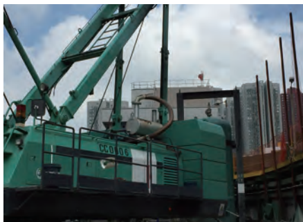
废气须经废气净化器过滤后才可排放到大气中 Exhaust gas filtered by exhaust-cleaning equipment before discharging to atmosphere
