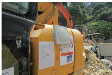
装设射频识别仪器探测附近是否仍有工人 RFID device installed to detect surrounding workers
