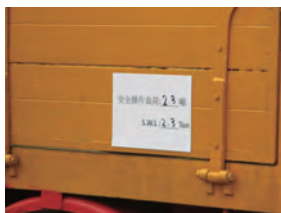
流动起重机上需标示安全操作负荷 Indication/markung of safe working load at mobile crane
