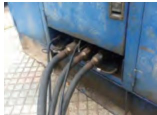
在压缩风喉加上套索 Compressed air hose fitted with whip check device
