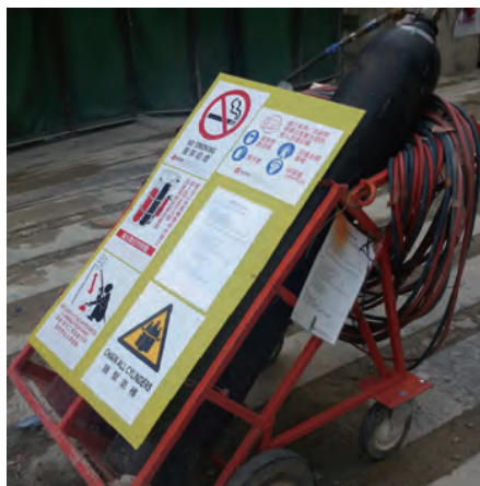
搬运大型圆形铁罐时，应使用适合的辅助工具 When moving metal drums, use a suitable handling aid
