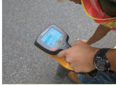
以手提探測器檢測地下公共設施的走線及其位置 Hand-held detector to check routing and locate for underground utilities
