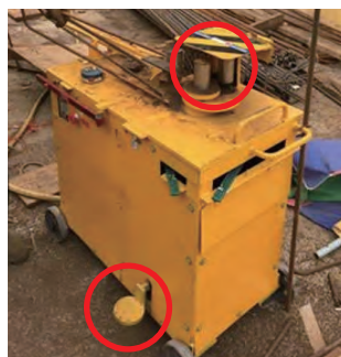
為屈曲鋼筋機器設置護罩腳掣和互鎖裝置。如無落下護罩，會截斷電源，停止機器的運作 Foot switch control and interlock guard on the bar bending machine. The device isolates the power supply to halt the operation, if guarding is removed
