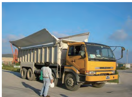
卸泥貨車配備的左右延展翼，減低物料意外地飛脫車身 Dump truck equipped with two covers to avoid debris accidentally coming out
