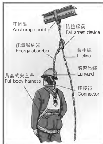
高空工作的個人抗墜防護系統 Fall protection system for working at height
