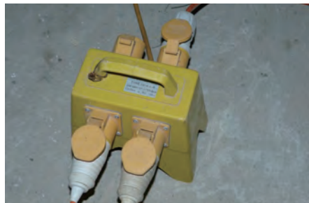
降壓變電器將高壓電降低至110伏特，適合一般手提電動工具使用 Step-down transformer provides 110V power supply source for use by hand-held tools
