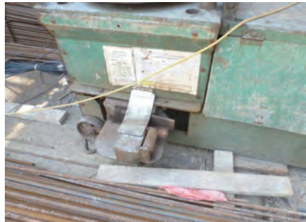
屈曲鋼筋機器需設置的護罩 Bar bending machine with guarding
