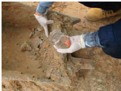
拆卸工程前，應取樣檢驗懷疑受污染的土壤：受污染的物质必須被移離 Prior to demolition, soil sample should be collected/ tested and the contaminated soil must be removed
