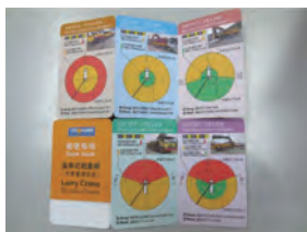
備有貨車式起重機的額定值降低圖，使安全操作負荷一目了然 De-rating chart of lorry-mounted crane gives quick guide on safe loading capacity
