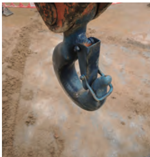
為吊鉤的安全扣加裝保險扣 Additional safety lock is added to the safety latch of hook
