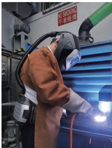
電弧焊接工須使用護盾、絕緣手套及圍裙 Welders should wear insulating gloves, handheld shield and apron
