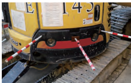
機尾安裝防撞棒 anti-collision rod at the rear of plant
