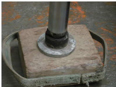
起重墊板的面積不得小於支重腳撐板的三倍 The lifting mat of area not less than 3 times of the float of the outrigger leg
