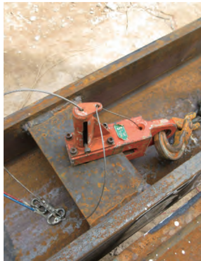
專為吊運字H字板樁用途的吊具 Tailor-made lifting gear for H-beam
