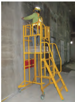
安全梯台於兩旁設置扶手 Step platform with handrails on both sides
