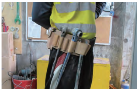
利用腰帶工具套穩妥地攜帶手提工具 Carry handheld tools securely with waist gear
