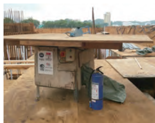
盛載木屑之容器 Receptacle below the cutting bench to receive sawdust
