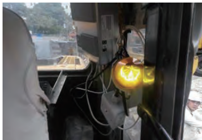
如有任何人員進入預設距離內的危險區域時，操作員便會接到警報 Operator is alerted when any personnel enters zone within a preset distance
