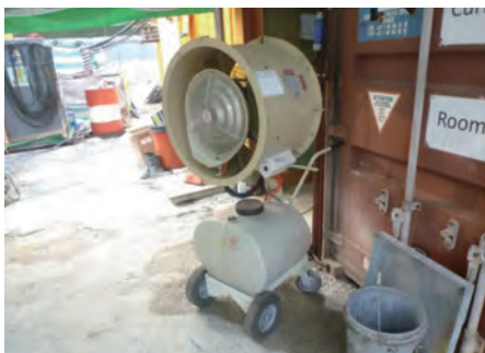
高容量的吹風機可使在工作間的工人更舒暢 Large blower with high air flow rate to workplace
