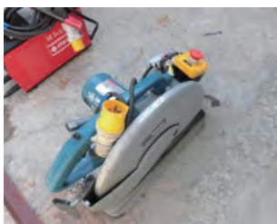
風車／圓鋸應設有護罩和緊急停止掣 Circular saw with guard and emergency stop
