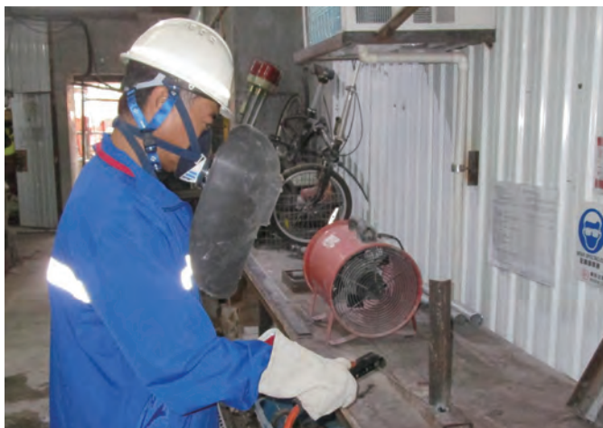
焊工穿上個人防護裝備方可進行焊接工作 Welders with personal protective equipment during welding
