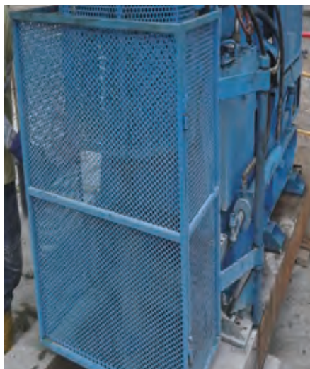
鑽機的活動部分必需設置護罩 Moving part equipped with shield guard
