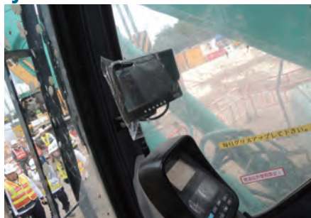
操作員透過閉路電視可觀察四周情況 Install CCTV system for operator to have a clear view of surrounding
