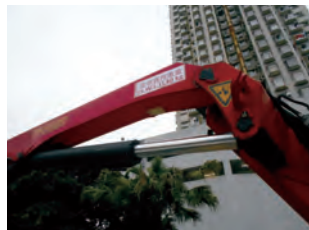
起重機上清楚標示安全操作負荷 Safe working load clearly marked on the crane
