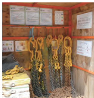
吊鉤及鈎環（塞古）妥善的存放 Proper storage of hooks and shackle
