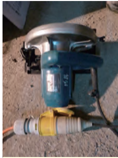
常用的雙重絕緣手提電工具 Double insulated hand-held tools commonly used for site works
