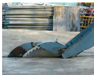
圓鋸上的護罩及鋸尾刀 Guard and riving knife on circular saw
