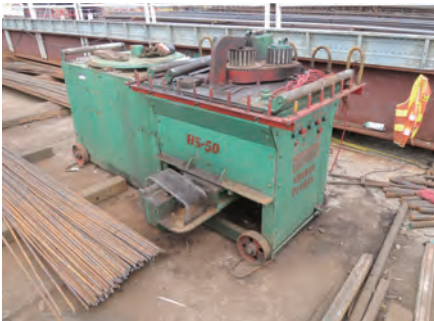
屈曲鋼筋機器需有足夠的工作空間 A typical steel bending machine on site with adequate working space
