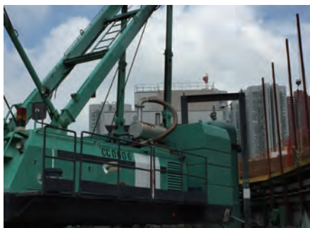
廢氣須經廢氣淨化器過濾後才可排放到大氣中 Exhaust gas filtered by exhaust-cleaning equipment before discharging to atmosphere
