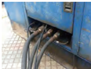
在壓縮風喉加上套索 Compressed air hose fitted with whip check device
