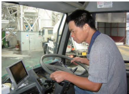
安裝閉路電視及螢光幕讓駕駛員清楚看見車輛後面的交通情況 Install CCTV and monitor for driver to have view of traffic at rear of vehicle
