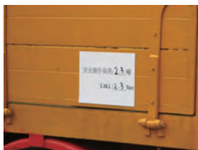
流動起重機上需標示安全操作負荷 Indication/markung of safe working load at mobile crane
