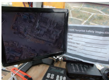
塔式起重機操作員藉閉路電視屏幕監察吊運區情況 CCTV system helps the tower crane operator to monitor the situation of lifting area
