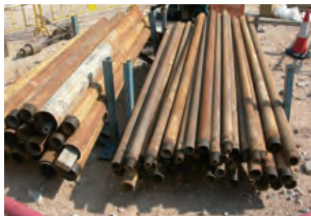
岩芯管和鑽杆應放在鋼架上 Stack core barrels and drill rods on steel frame trestles
