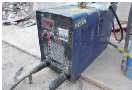
焊機殼必須接地（帶電部份需要有絕緣保護） Shield of welding machine - Earthed (Live conductor terminals should be insulated)
