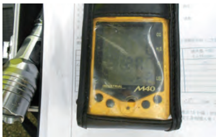
A calibrated gas detector used to measure the concentration of poisonous/flammable gases inside a confined space
