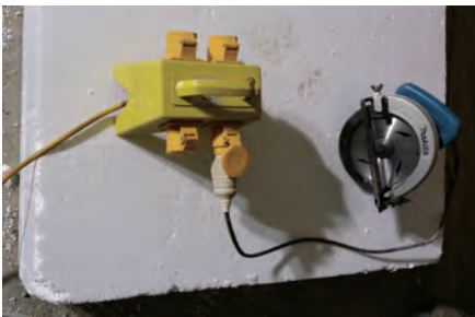
降壓變電器將高壓電降低至110伏特，適合一般手提電動工具使用 Step-down transformer provides 110V power supply source for use by hand-held tools
