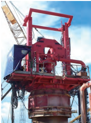
大口徑鑽孔樁一般涉及的機械 Plant and equipment used in large diameter bored pile construction
