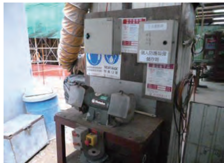
為砂輪機設置護罩和在當眼處張貼安全海報／告示 Abrasive wheel with guarding and relevant notice/poster is posted at the location
