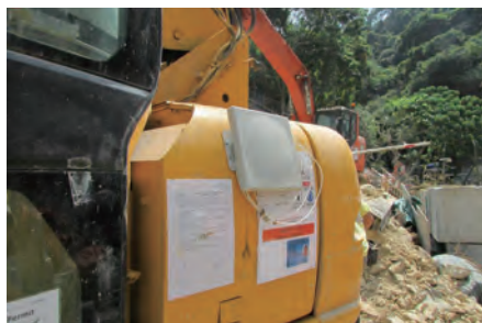
裝設射頻識別儀器探測附近是否仍有工人 RFID device installed to detect surrounding workers
