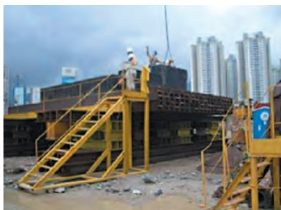
Final set up of mass steel kentledge
