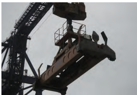
Attached working platform for maintenance of lifting spreader and lifting block of crane operation
