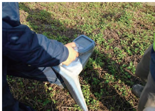
Pipe and Cable Locator
