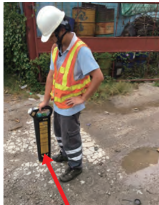
Electronic device to locate underground utilities
