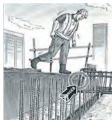
Injury caused by falling on unprotected protruded steel bars Protection of workers from injury using one of the protective options
