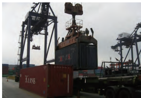
Attached working platform for maintenance of lifting spreader and lifting block of crane operation
