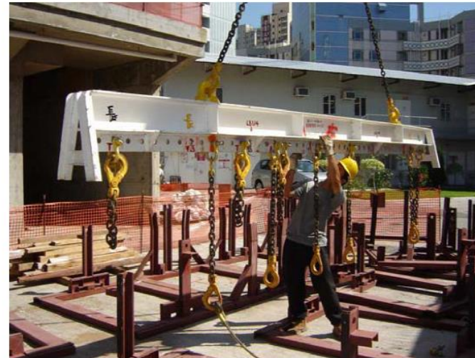
Loading Test to lifting beams for precast elements
