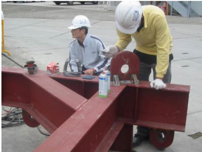
Welding Test on Lifting Points of Lifting Gears
