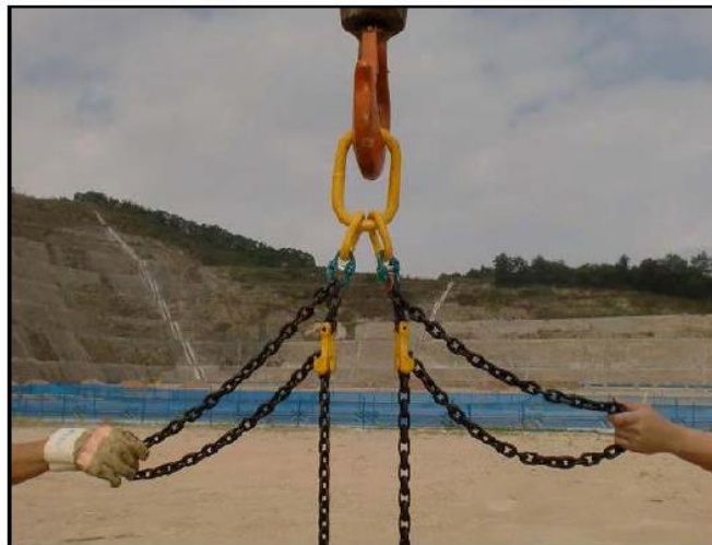
Shortening clutch connected to chain in the normal direction
