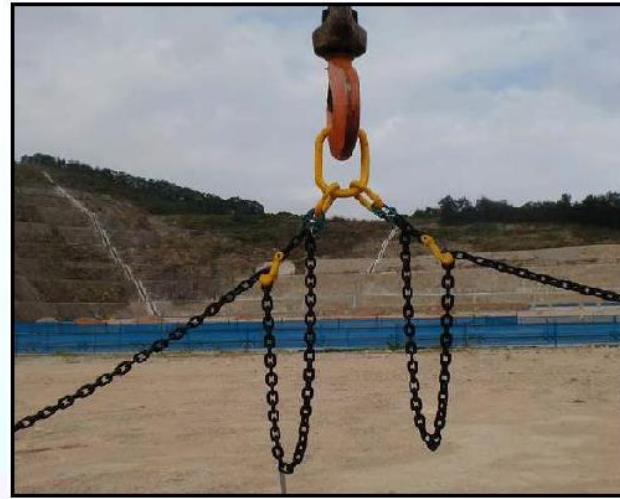
Shortening clutch connected to chain in the reverse direction
