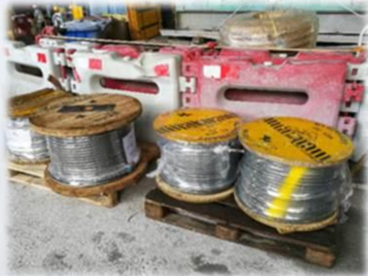
New Wire Ropes for Tie bars and Lifting Section
