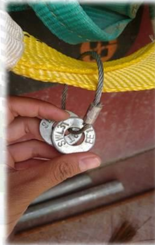
Provision of Double Marking of Lifting Gears & Nylon Webbing Slings (Prohibition of re-examining the used nylon webbing slings) 20
