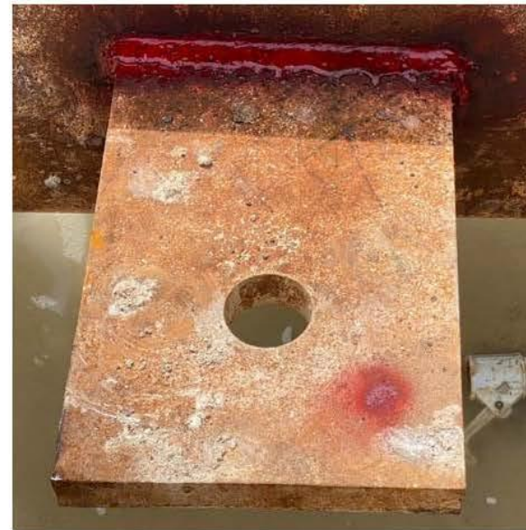
Checking Method of Lifting Eyes 吊眼檢查方法
