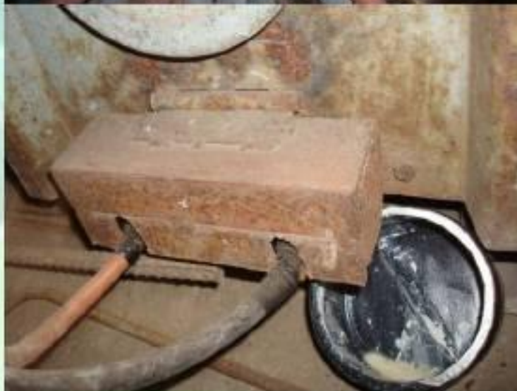
Improper insulation and protection of welding cables
