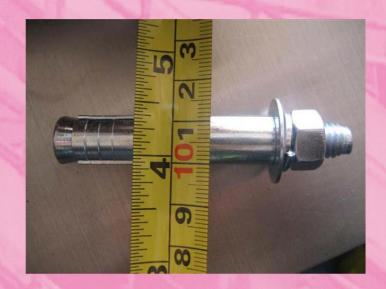
Checking of Anchor Bolt Size (≥12mm ø)
