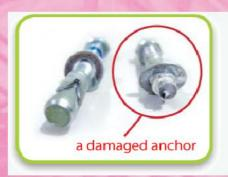
Diagram 6: The structure of the anchor bolt was seriously damaged (The right-hand side anchor bolt) as a result of fixing it with too large tightening torque.
