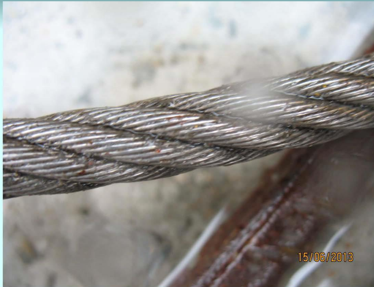
Wire rope showed no severe abrasive wear
