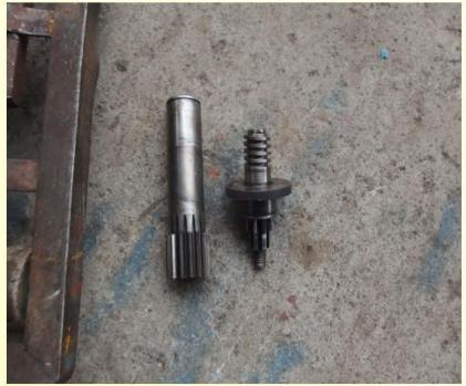
Safety Lock (centrifugal type) fails to protect SWP from excessive tilting in slow failing e.g. gear box failure, dead man switch malfunctioning
