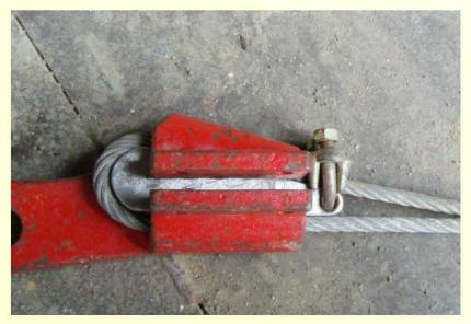
Hand tools are slow and no measurement of tightening torque
