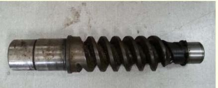
Excessive wear and tear of sun gear lead to gear box failure
