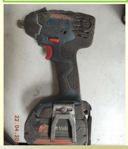
IP 44 weather proof insufficient protection against ingress of water
