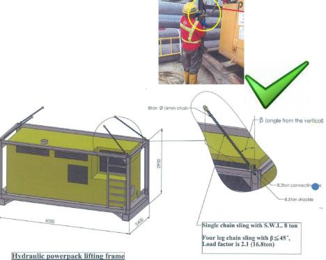
Adding bridging chains on the 4 corners of steel frame to eliminate workers to work at height while rigging. This device would allow workers rigging on ground and reduce the chance to work-above ground. It can effectively eliminate the risk of working at height while rigging.
