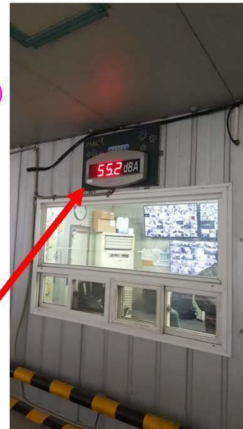
Display of Air Pollutant & Noise Monitoring Readings (at hoarding outside site)
