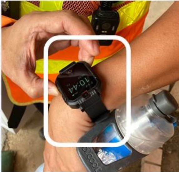
The worker worn the smart switch for monitoring health status
